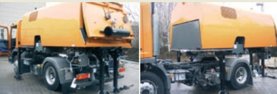
Mounted on various makes of chassis , Bucher Schörling's quick-change frames allow the sweeper or salt spreader body to be switched in a matter of minutes. This means the carrier vehicles can be in constant use, thus providing a fast payback. Vehicles and their bodies are available from one source, all assembled and serviced by Bucher Schörling.
